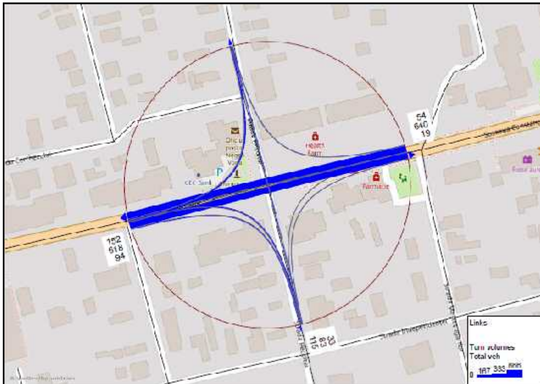
Figure 3.19. Measured values (physical vehicles) Station 2, time interval 06:30 - 19:30.
