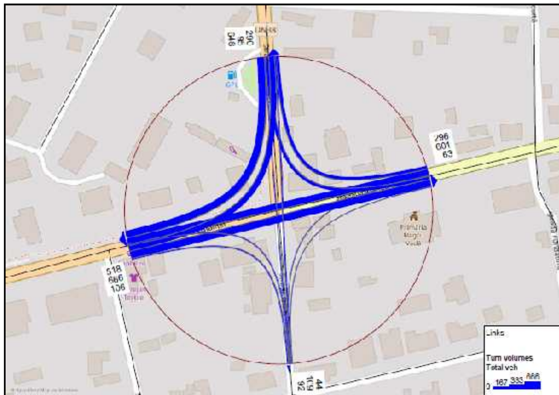
Figure 3.17. Measured values (physical vehicles) Station 1, time interval 06:30 - 19:30.
