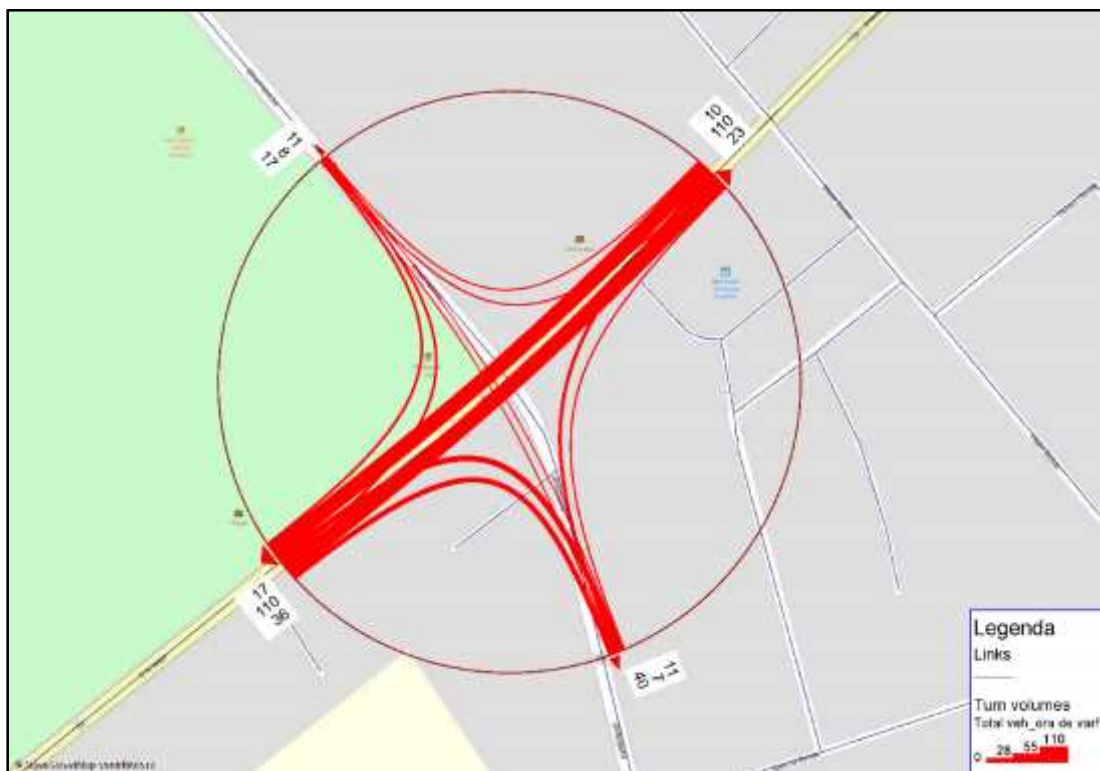
Figure 3.28. Measured values (physical vehicles) Station 1, rush hour traffic.
