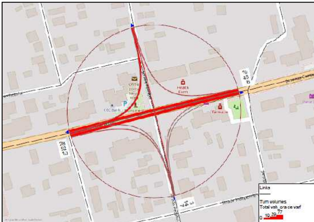
Figure 3.20. Measured values (physical vehicles) Station 2, rush hour traffic.
